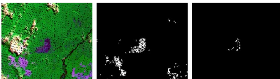
Figure 9. Under-detection by E1 in the Brazilian forest in July. (left) The burnt areas can be seen on the ATSR image. (center) They are detected by the K1 algorithm but missed out by (right) the E1 algorithm.
